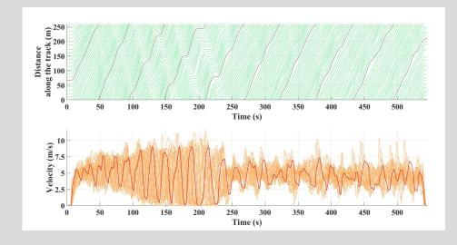
Human driving leads to traffic waves with oscillatory velocity profile but acceleration are bounded within  $\pm~0.5~\text{m/s}^2$
