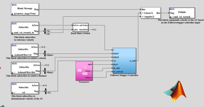
Code-generation method allowed us to design controller at block level while reducing debug time. Additionally, we didn't need to write separate code for simulation and hardware-implementation in real autonomous vehicle. This further cuts overall design time.
